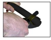
**4** Chamfer end of pipe using <u>Continental's ID</u> <u>chamfering tool with ID</u> <u>gauge</u>.
